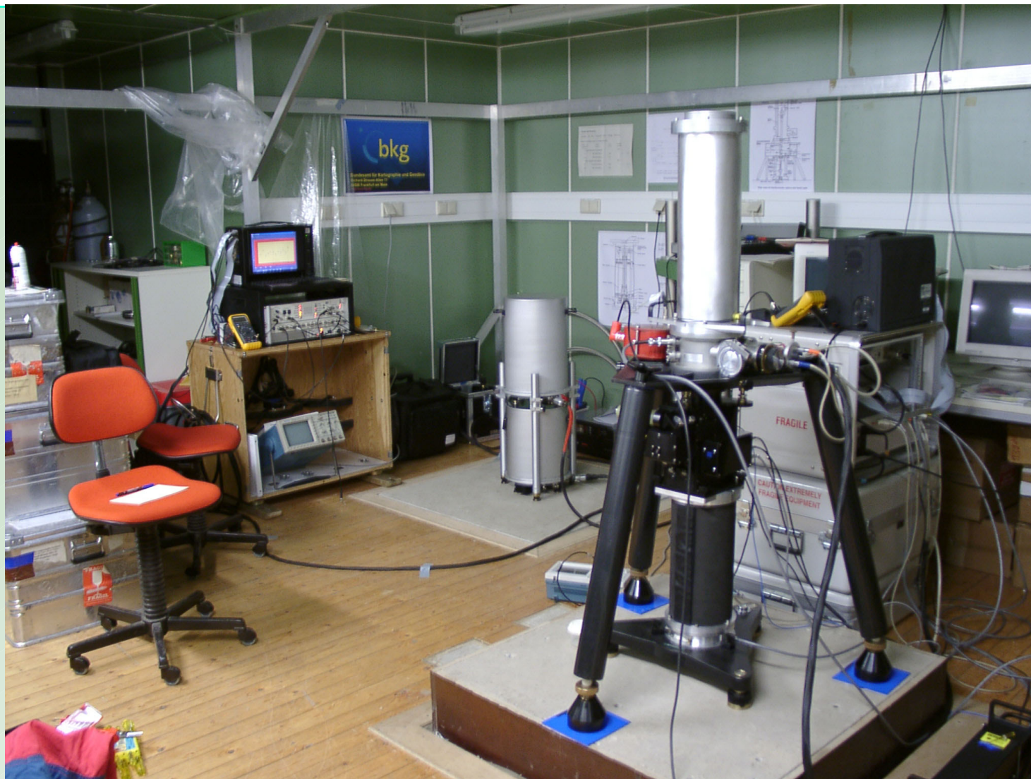
Bad Homburg gravimetric observatory, pillar BA with A10 #002 and pillar AA with FG5-101
